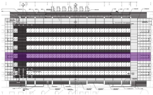
Figure 23: Steel Erection for 5 th floor at night, metal decking installed, and concrete poured during day. Prefabricated MEP systems installed on 2 nd floor.
