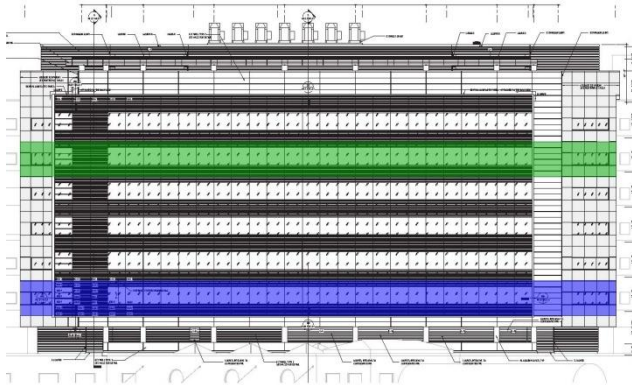
Figure 14: As the steel strengthening work moves to the 3 rd floor, the move out process will continue to the 7 th floor.
