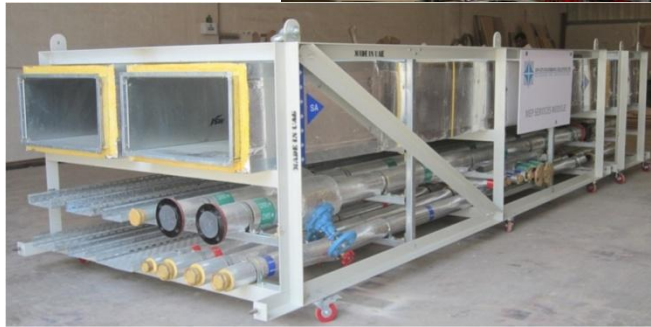
Figure 52: Prefabricated MEP Rack
