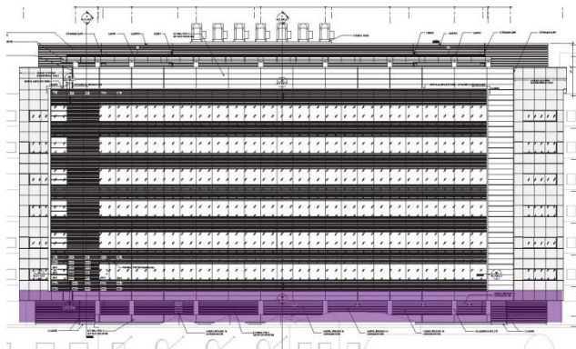
Figure 20: The 2 nd floor stub columns will be installed and the building pad will be prepared.
